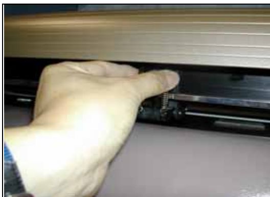
Figure 2-15 Correct way to move pinch rollers
